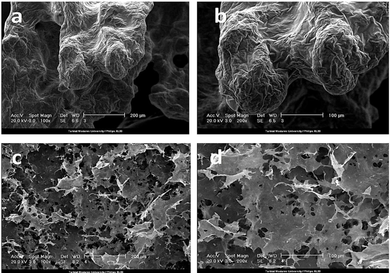
**Figure 1.** Scanning electron microscopy images of (a, b) the microencapsulation matrix and (c, d) microencapsulation matrix treated under gastrointestinal juices.
