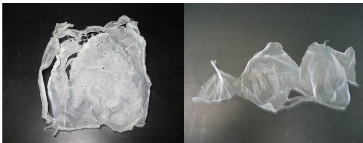
Figure 2. Cast films of PHBHV extracted from H. pseudoflava biomass cultivated on hydrolyzed whey permeate (own pictures of the authors)
