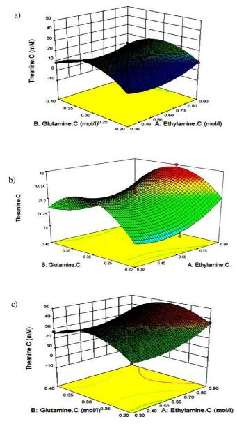
**Fig. 5.** Three-dimensional plots for theanine concentration vs. ethylamine and L-glutamine concentration with the enzyme solution volume of (a) 1 ml; (b) 3 ml and (c) 5 ml.
