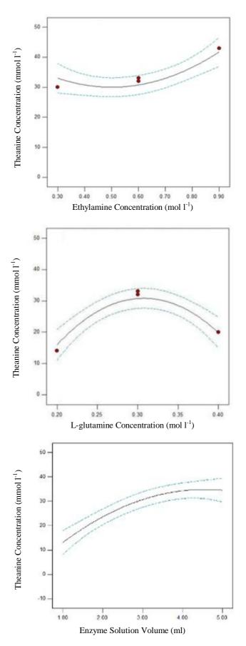
**Fig. 7.** Theanine concentration vs. (a) Ethylamine concentration; (b) L-glutamine concentration and (c) enzyme solution volume.
