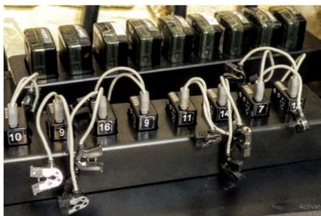
**Figure 1.** Eight-Channel Electromyography Noraxon Device.
