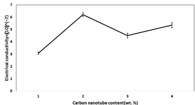
**Figure 5.** Electrical conductivity of the prepared scaffolds with different CNT content.
