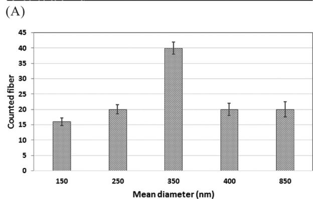
**Figure 2.** (A) SEM micrograph and (B) Fiber mean diameter distribution of the prepared sample with 4 wt. % of CNT.
