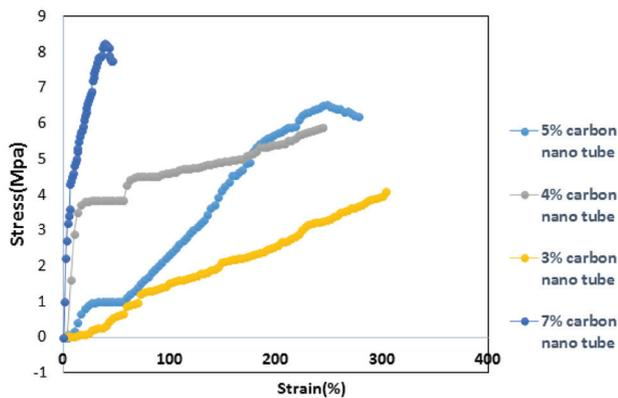
Figure 6. Stress-Strain curve of the prepared scaffolds.
